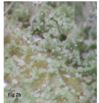
Small particulate airborne debris (<1mm) in factory environment deposited on a glue trap.
