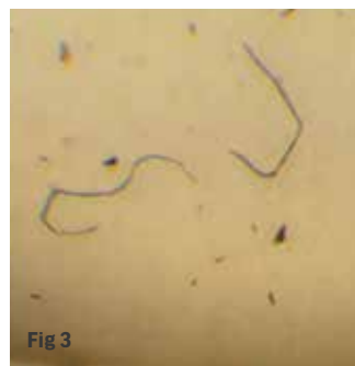
Fig 3 & Fig 4 Showing microscopic fibres in the environment detected on glue boards
